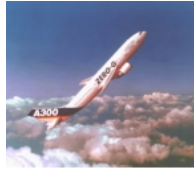
FIG. 2: Parabolic maneuver of the airbus A300 Zero-G.
